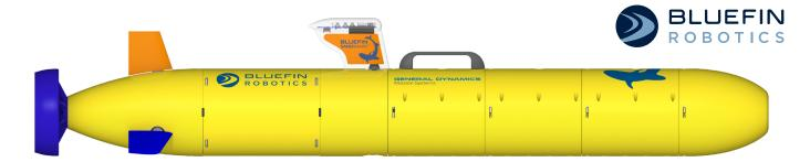
The Bluefin SandShark® is a one-person-portable, low-cost autonomous underwater vehicle (AUV) designed to leverage today's miniaturized sensors and also be the development platform for the next generation.
