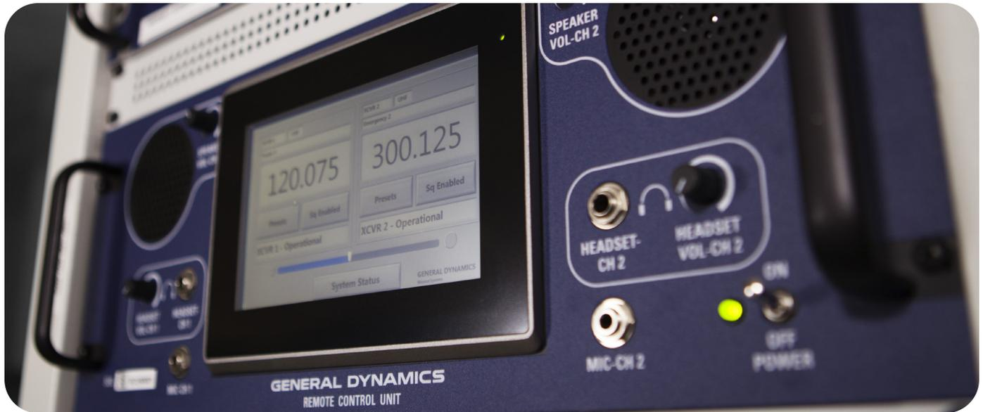
Remotely control up to two remote CM-300/350 (V2) transceivers over a network connection
